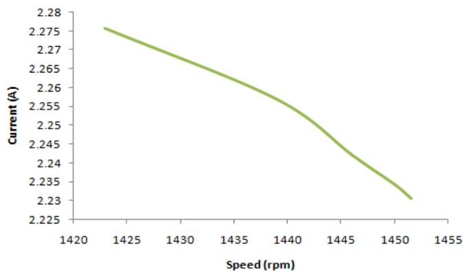
Fig. 9: Current-speed characteristics of the motor on load using CCPM
