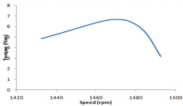
Fig. 8: Torque-speed characteristics of the motor on load using CCPM
