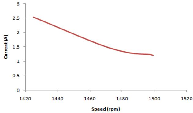
Fig. 7: Current-speed characteristics of the motor on no-load using CCPM
