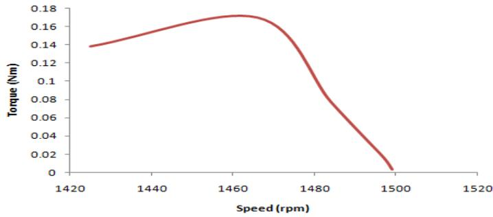
Fig. 6: Torque-speed characteristics of the motor on no-load using CCPM
