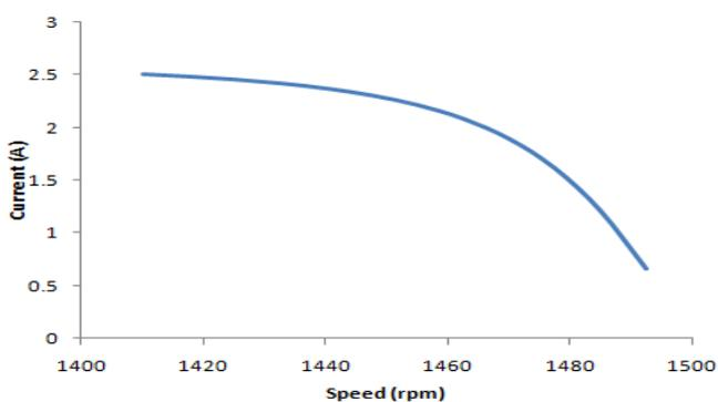
Fig. 5: Current-speed characteristics of the induction motor on load using FEMM
