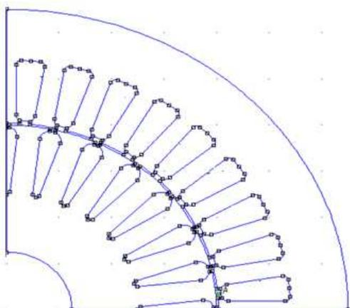
Fig. 2: One pole-pitch section of the motor
