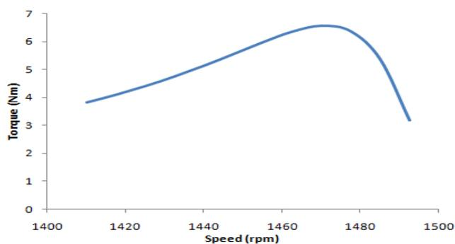
Fig. 4: Torque-speed characteristic of the induction motor on load using FEM Version 4.0
