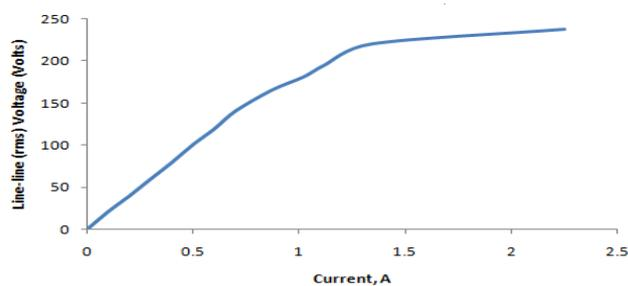
Fig. 3: No-load (open-circuit) characteristic of the induction motor
