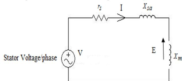
Fig. 1: Equivalent Circuit of Induction Motor on No-Load
