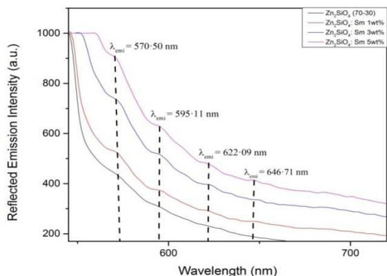
Figure 5. Emission spectra of (70-X) Zn<sub>2</sub>XSm<sub>30</sub>SiO<sub>4</sub> at X = 0, 1, 3 and 5 wt%
