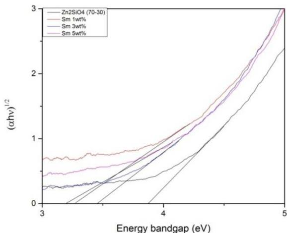
Figure 2. Optical band gap of (70-X) Zn<sub>2</sub>XSm<sub>30</sub>SiO<sub>4</sub> at X =0, 1, 3 and 5 wt%
