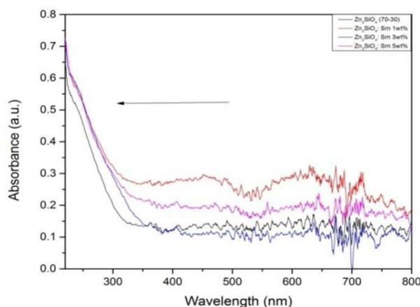
Figure 1. Absorption spectra of  $(70-X)\text{Zn}_2\text{XSm}_3\text{SiO}_4$  at  $X = 0, 1, 3$  and  $5$  wt%
