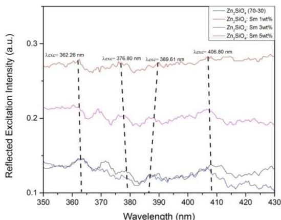
Figure 4. Excitation spectra of (70-X) Zn<sub>2</sub>XSm<sub>30</sub>SiO<sub>4</sub> at X = 0, 1, 3 and 5 wt%
