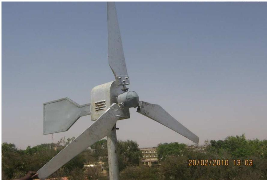
**Plate 1:**The Complete Assembly of the Wind Turbine Constructed
