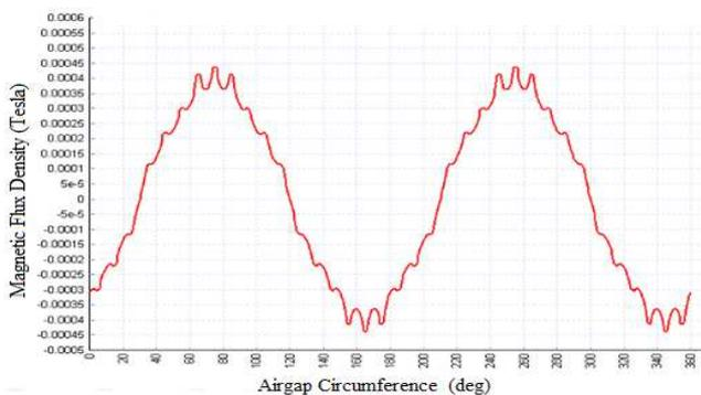
Fig. 3: Magnetic Flux Density Distribution in the Air-gap
