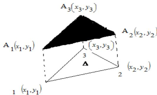
Fig. 2: Linear interpolation of the potential function  $A_n$  in the n-th triangular element
