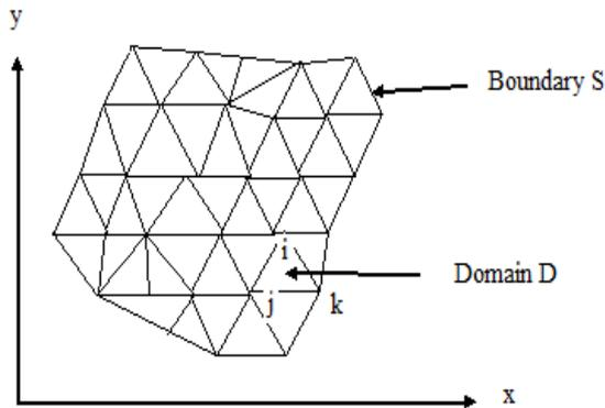
Fig. 1: Discretization of the field region by triangular finite element
