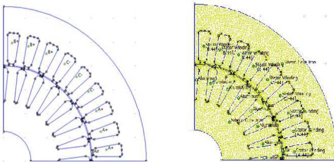
Fig. 4: 2-D Model (a) One-Quarter of the Motor Geometrical Drawing and (b) Motor's associated generated mesh.
