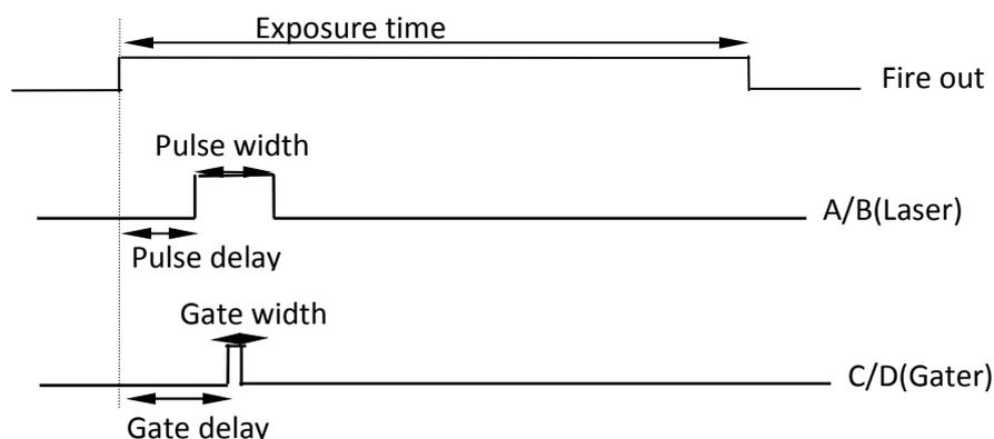
Figure 3: Schematic of the timing diagram of the SRS delay generator.
