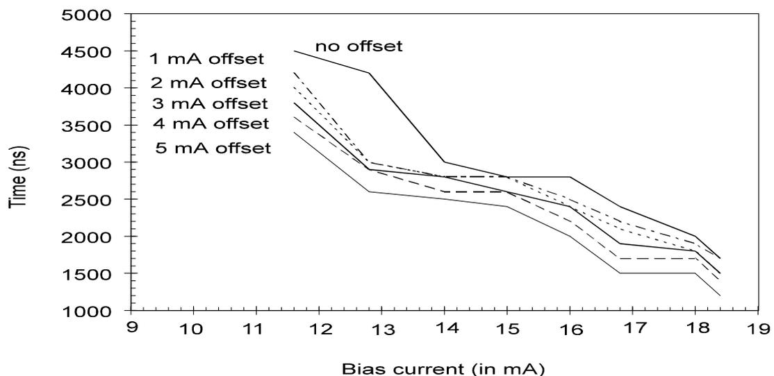
Figure 8: Time required in attaining stable state versus dc-bias currents.
