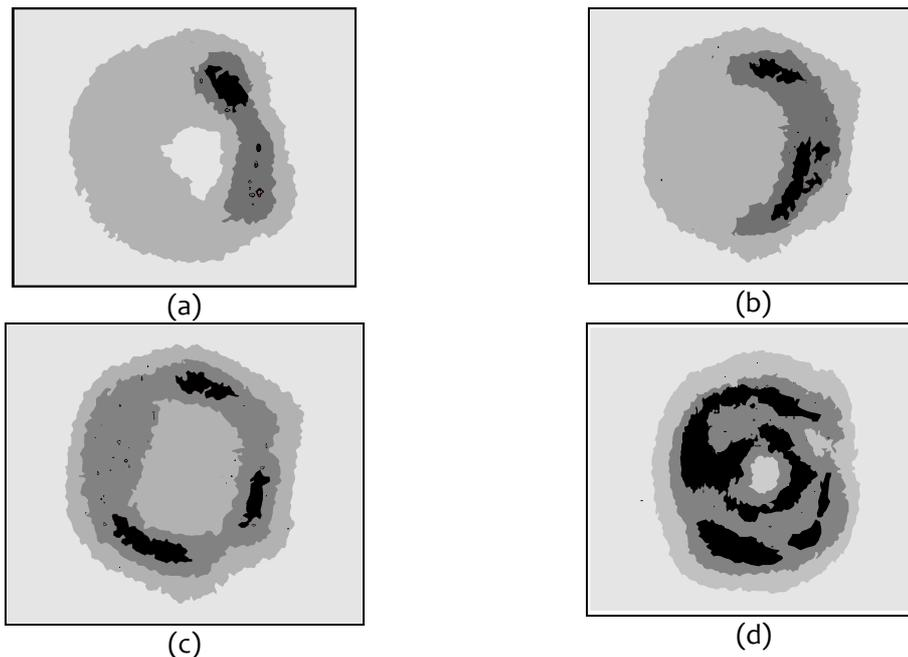
Figure 7 Formation of optical filaments due to carrier guiding and mode partitioning at I=15 mA, (a) 30 ns, (b) 50 ns, (c) 250 ns, (d) 3μs.
