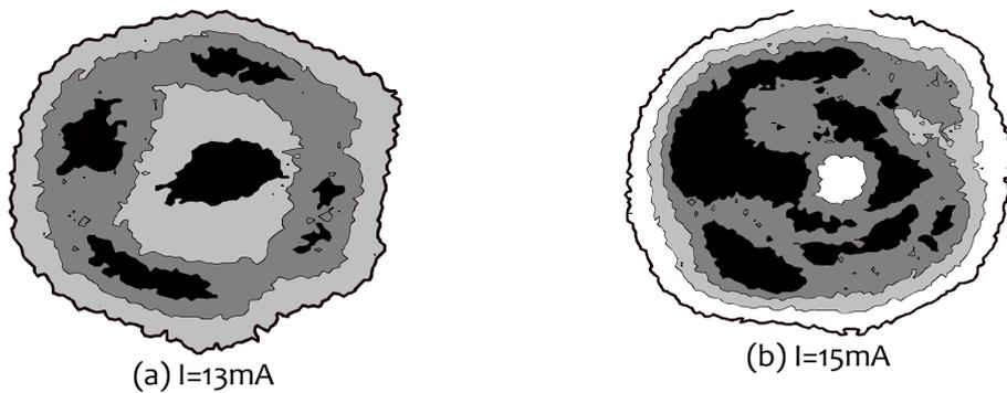
Figure 5: Steady state near-field patterns for bias currents of (a) 13mA and (b) 15mA.
