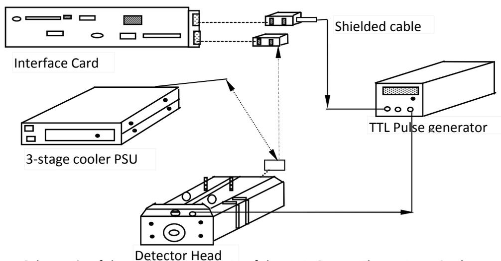
Figure 1: Schematic of the main components of the InstaSpec V Three stage Cooler system.
