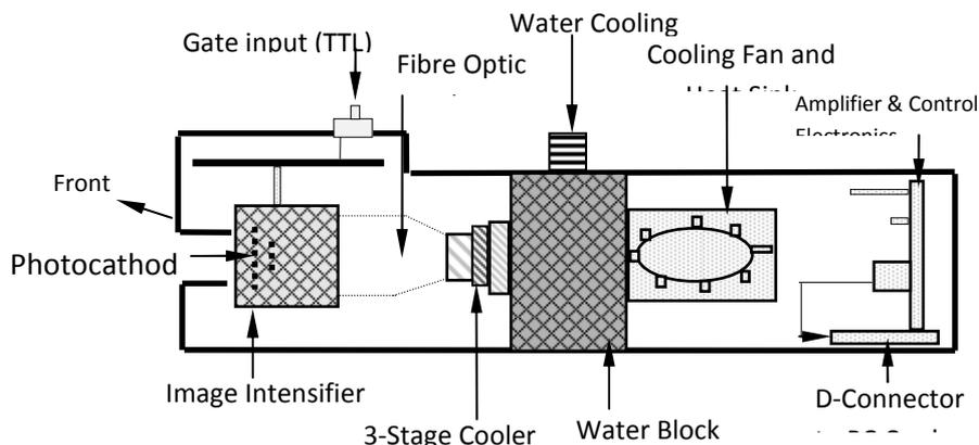
Figure 2: Schematic of the ICCD-camera Head [Oriel Instruments, (1996)]
