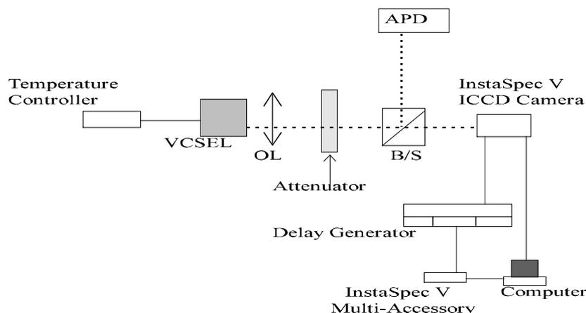
Figure 4: Schematic for the experimental set-up; OL is a microscope objective lenses, B/S is beam-splitter.
