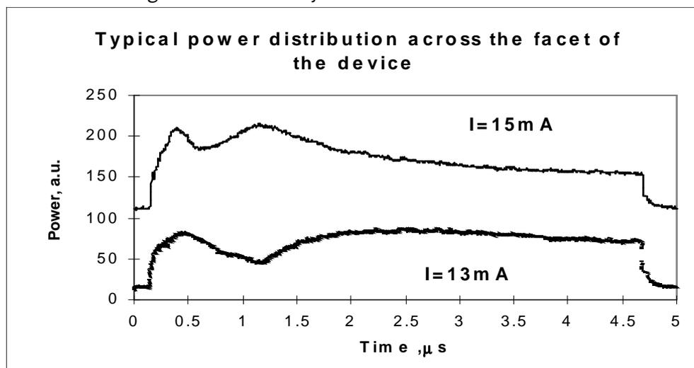
Figure 6: Si-APD response showing the total power of the mode partition development due to optical filaments.
