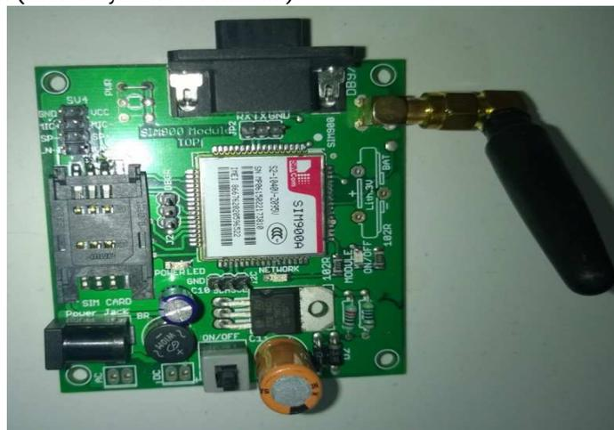
Figure 5: GSM Modem (original picture)
